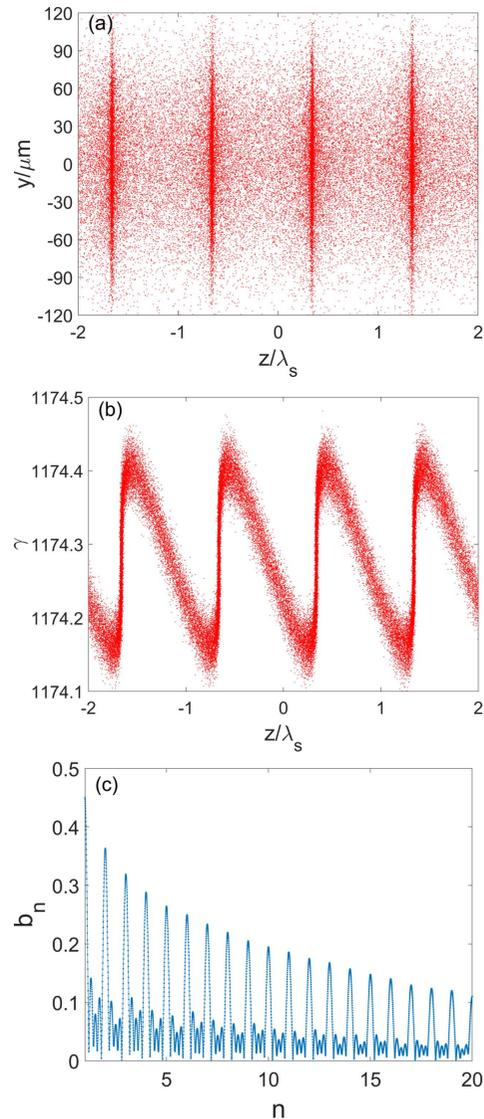
**Figure 5** Simulation results of (a, b) the microbunching distribution and (c) bunching factors at various harmonics after the laser-beam interaction of ADM.  $\lambda_s$  is the seed laser wavelength.
