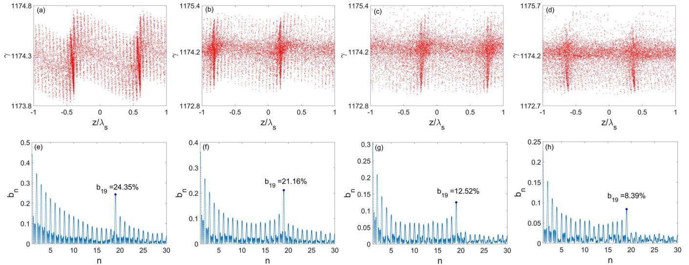
**Figure 9** Simulation results of the longitudinal phase space (top) and bunching factors at various harmonics (bottom) at the exit of the first bending system [(a) and (e)], the second bending system [(b) and (f)], the third bending system [(c) and (g)] and the fourth bending system [(d) and (h)].  $\lambda_s$  is the seed laser wavelength.
