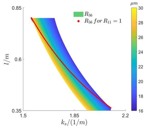
**Figure 3**  $R_{56}$  values at different  $k_s$  (the square root of the focusing quadrupole's strength) and  $l$  (the length between the centers of the bends and the quadrupoles). Here, the red dots represent  $R_{56}$  values calculated using the corresponding  $k_s$  and  $l$  when  $R_{11}$  is equal to 1.
