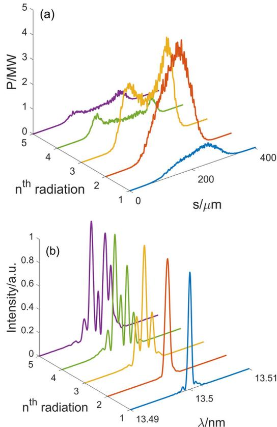
**Figure 8** Radiation pulses (a) and spectra (b) at the exit of five radiators (3.75 m).
