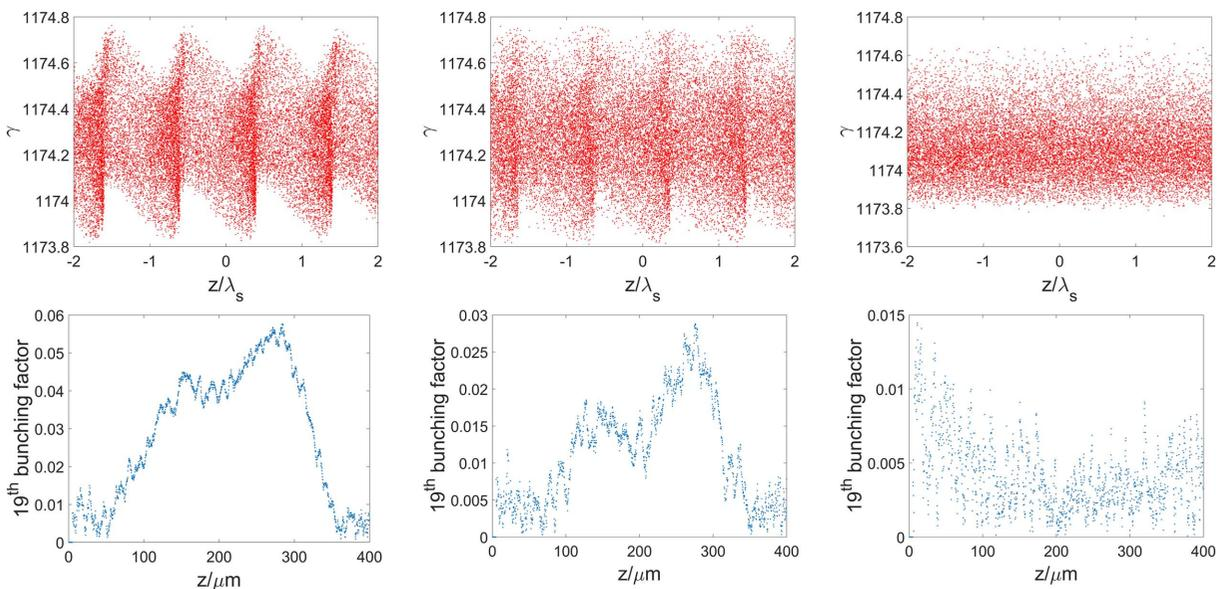
**Figure 10** Simulation results of the longitudinal phase space (top) and 19th bunching factors (bottom) along the beam at the exit of the first-order four-bend achromat with  $R_{56} = -10 \mu\text{m}$  (left), the first-order triple bend achromat with  $R_{56} = 16 \mu\text{m}$  (middle) and the first-order isochronous achromat (right).  $\lambda_s$  is the seed laser wavelength.
