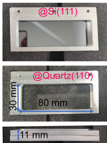
Figure 5 Top and side views of the photographs of Laue analyzers. The top panel depicts silicon (111) and the middle panel depicts quartz (110). The aperture size is 80 mm in the bent direction and 30 mm in the non-bent direction. The bottom panel shows a side view of the bender frame. The crystal curvature of \sim 150 cm is visible.
