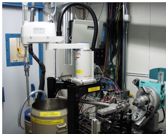
Figure 3 Photograph of the first robot installed on SSRL BL7-1 ca. early 2000s. The robot mimicked many of the manual operations developed for manual cryocooling and became the basis for fully automated sample handling under cryo-conditions.
