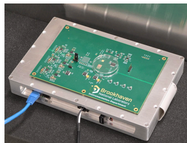
Figure 7 Photograph of the detector with the 3FI ROIC – before sensor assembly.
