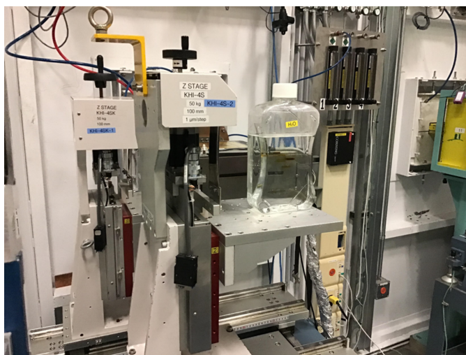
Figure 5 Tank of water used as an incident beam spectral flattening filter, upstream of the crystals.
