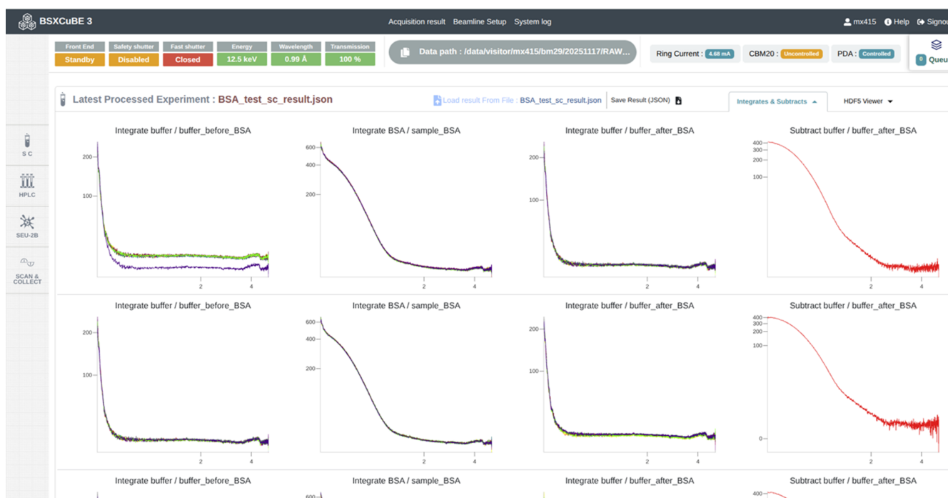
Figure 9 BSxCuBE-Web GUI representation of data processing results from FreeSAS (Kieffer et al. , 2022).
