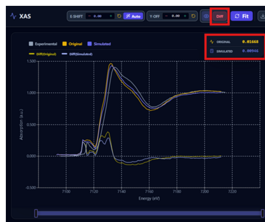
Figure 6 Difference spectrum and R -factor diagram.
