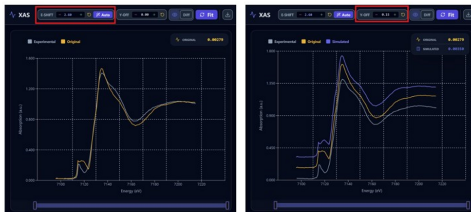
Figure 5 E-SHIFT and Y-Offset function diagram.
