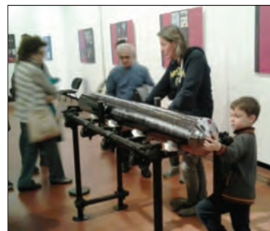
“The rocket”, a silicon single crystal of 250 kg grown by the Czochralski method.
